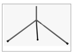
**STEP 2:** Insert Top Pole (C) into Tripod (B) top until push-pin snaps into place. Tighten Thumb Screw in threaded nut attached to opposite side of the push-pin hole.
