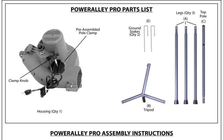
**STEP 1:** Slide Legs (A) into Tripod (B) base until push-pin snaps into place.
