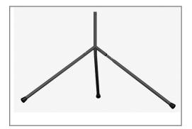
**STEP 2:** Insert Top Pole (C) into Tripod (B) top until push-pin snaps into place. Thread Thumb Screw (D) into threaded nut attached to opposite side of the push-pin hole.
