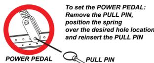
**NEVER adjust the POWER PEDAL when the THROWING ARM is pulled back and locked into position.**
