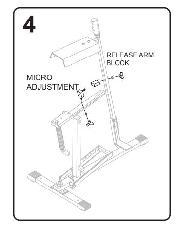
4) Attach the MICRO ADJUSTMENT and the RELEASE ARM BLOCK into the numbered hole based on the desired speed shown on the chart located on the TOP SHIELD of your machine.
