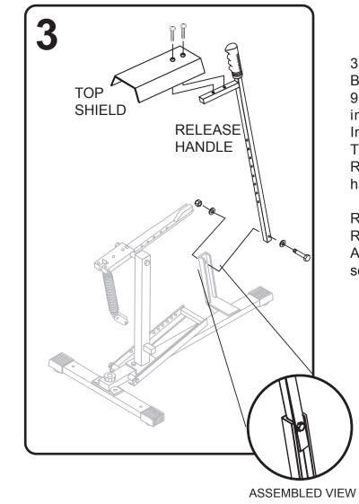
3) Remove the nut, bolt and two washers from the BASE ASSEMBLY shown in diagram 3 with two 9/16" wrenches. Align RELEASE HANDLE to the inside the "U" channel of the BASE ASSEMBLY. Insert bolt and washer and attach washer and nut. Tighten secure but **DO NOT OVER TIGHTEN.** The RELEASE HANDLE should move freely but not have side to side movement.
