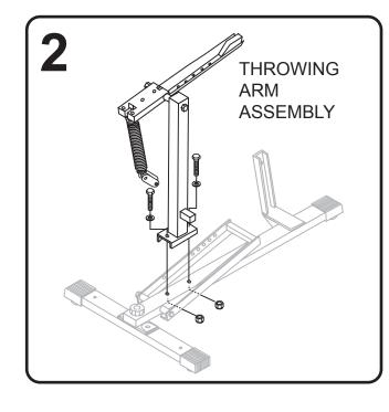
2) Remove the nut, bolt and washers from the THROWING ARM ASSEMBLY shown in diagram 2 with two 9/16" wrenches. Align the THROWING ARM ASSEMBLY to the BASE ASSEMBLY. Attach the two bolts and washers and tighten. (The bottom plate on the BASE ASSEMBLY is threaded). After the THROWING ARM is tightened to the BASE ASSEMBLY reattach the nuts and tighten securely.
