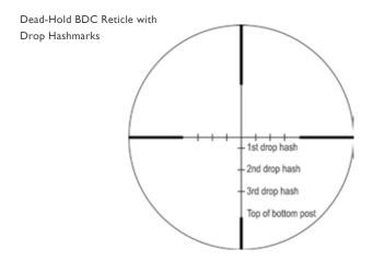
This model of Vortex riflescope uses the second focal plane design—the listed BDC yardages will only be valid with the riflescope set at the highest magnification.
