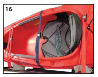
Install the blue safety strap around the center of both kayaks. This is easiest done by holding the buckle and throwing the free end over the top of both kayaks. Dress the free end back under the kayaks, and, up and through the buckle. Pull down to tighten. See image 16.
