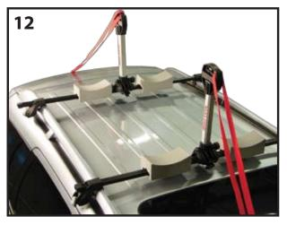
. Place the strap loops parallel to the carriers with the front strap loop on the windshield and the rear strap loop on the back of the vehicle. See image 12.
