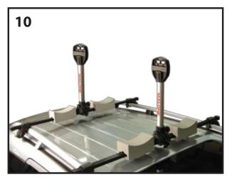
Raise the carriers to the up-position and confirm alignment. Tighten the t-knobs until both carriers are securely fixed to the cross bars. Place foam blocks onto the cross bars and next to the carriers. See image 10.
