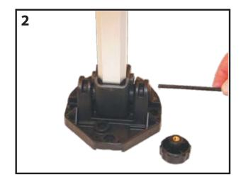
. With the holes in the base and post aligned, push the bolt through the two assemblies until the end of the bolt is exposed.
