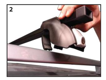
Place Cross Bars onto the vehicle's raised side rails. Adjust for the load to be carried. Note: Bars must be separated by a minimum of 24". See image 3.
