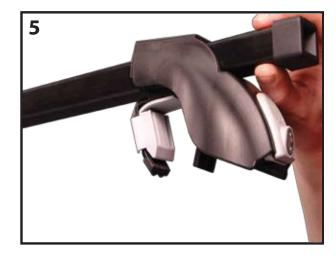
Insert the Installation Wrench and tighten the bolt clockwise until the feet hold the cross bars firmly in place. Apply pressure to confirm that no movement of the Cross Bars can be felt. Raise the lock plate and lock with Key. See image 6.
