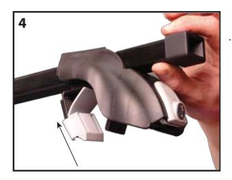
Push the Rubber Spacer Block up each foot until the top flat section is formed around the top of the foot. See image 5.
