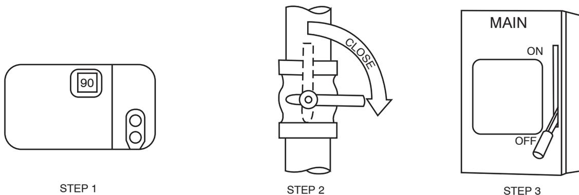
Fig. 7 - To Shut-off Unit Electric Cooling
