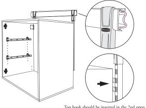
Top hook should be inserted in the 2nd open notch from the gripper on the inside row of notches.
