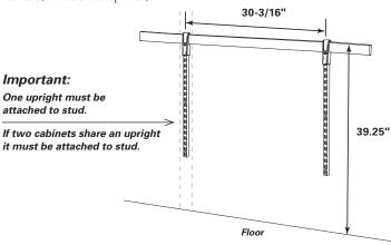
HAZARD: If upright is not attached to stud, the load claim is null and void.
