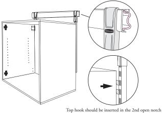
from the gripper on the inside row of notches.
