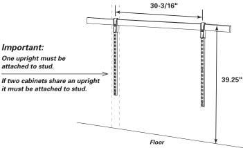
HAZARD: If upright is not attached to stud, the load claim is null and void.
