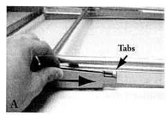
Install Brackets onto the left and right side of Frame. Slide the nose of the Bracket into tabs on Frame (as pictured above). The nose of the Bracket should be facing the chrome tube on the front of the Frame.
