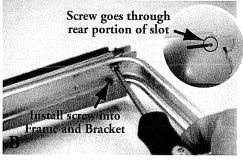
Place washer onto screw and install screw through Frame and into Bracket Do not fully tighten screw. Repeat for opposite side. Note: Screw should insert through rear portion of Bracket slot.
