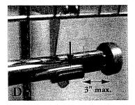
After expanding Clothes Rod to desired length, place into Rod Hangers and press down to snap into place. Note: Do not extend more than 3" past Rod Hangers.
