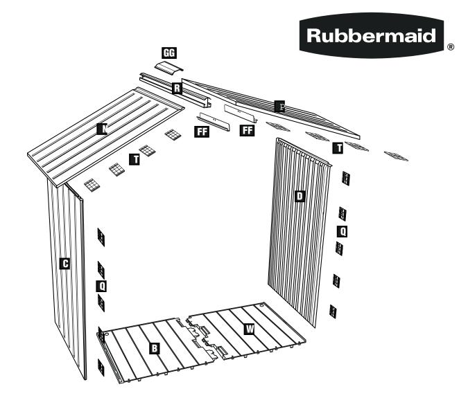
• Only 1 Extension Kit should be added to a Big Max Junior or a Big Max Shed. • These instructions can be used to assemble a Big Max Extension Kit to a Big Max Junior or a Big Max Shed. All the illustrations show the Big Max Extension Kit being assembled to a Big Max Shed.
