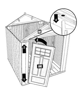
Install Right Door Panel (AF) inserting the lower hinge pin into Front Right Floor (U) socket, lift the right end of the Gable (M) enough to insert the top hinge pin on Right Door Panel (AF) into the Gable (M) socket.
