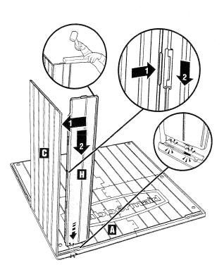
Using a screwdriver, punch out the screw holes on the top of Left Side Panel (C) 2 Places. Align lap joint between Left Side Panels.
