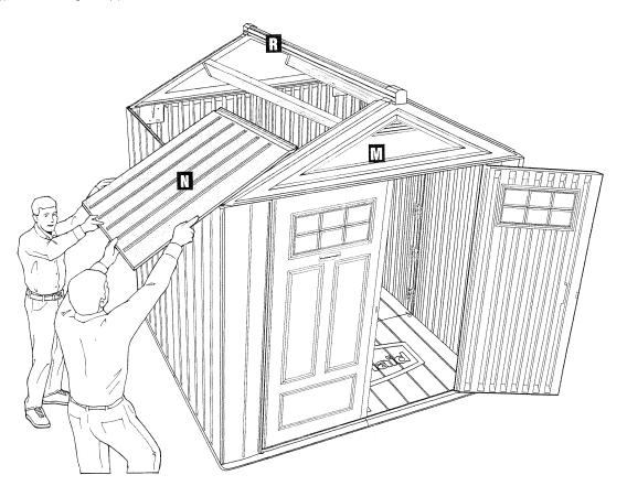
Using (2) step stools (1 inside shed, 1 outside shed), lift bottom of the roof panel above horizontal, guide the roof panel into the Ridge Beam (R), align the front Gable (M) rib with the channel in Left Roof Panel (N), engage Left Roof Panel (N) in Ridge Beam (R) by lowering the bottom of the roof panel onto the shed assembly (hold Ridge Beam (R) to prevent twisting). DO NOT SNAP ROOF DOWN.
