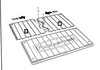
Caution: When installing screws do not overtighten.
