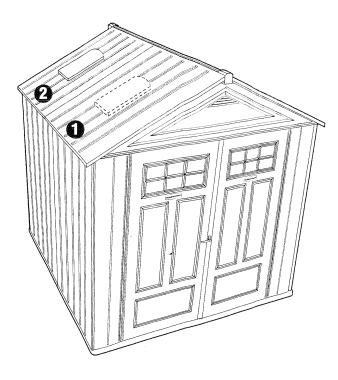
The Skylight Roof Panel can be assembled in 1 of 2 different positions Assembly instructions show the Skylight Roof Panel being assembled in position 2.
