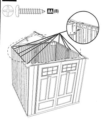
Caution: When installing screws do not overtighten.
