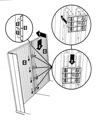
Lubricate dovetails on Left Back Panel (E) 4 places with liquid soap. Connect Left Back Panel (E) into dovetails of Left Side Panel (C), engage snaps on bottom of Left Back Panel (E) into Back Left Floor (B).
