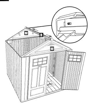
Align slots in Ridge Beam (R) with holes in Gable (M) tabs, install Bolt (BB), Washer (CC), and Nut (DD) 1 place, **ONLY TIGHTEN NUT 'FINGER' TIGHT**.
