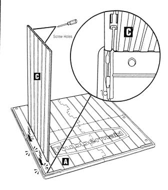
Caution: When installing screws do not overtighten.
