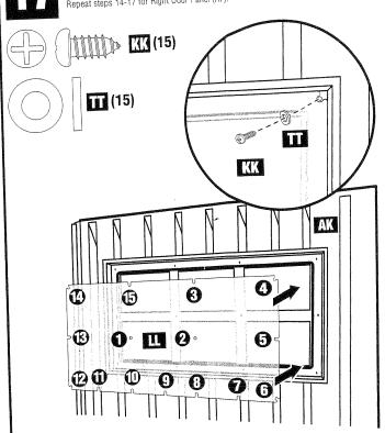
Caution: Tighten screws only enough to compress gasket.
