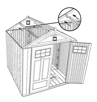
Note: Highly recommended for areas of externe snow or extreme heat. Usage of the lumber supports is optional. The Big Max Shed is designed to function properly without them; however, the lumber provides extra roof support in extreme conditions.
