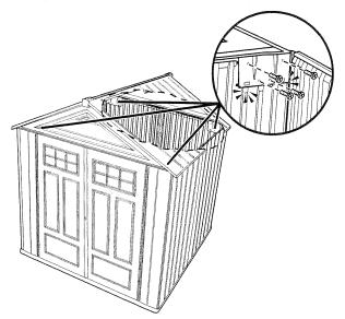
Caution: When installing screws do not overtighten.
