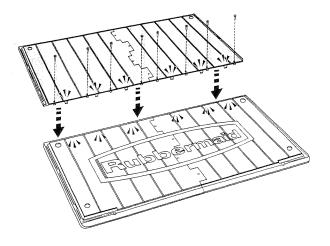
Using a screwdriver, punch out the screw holes on the top of Left Side Panel (C) 2 Places. Connect Left Side Panel (C) into Front Left Floor (A).
