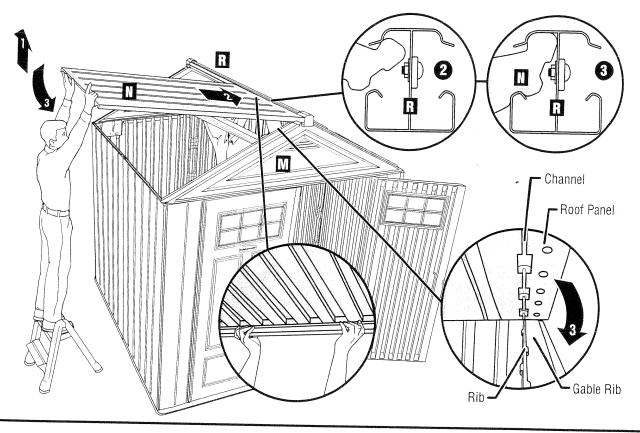
Lubricate roof snaps on Back Gable (M) 8 places. Raise the Left Skylight Roof Panel (AN) onto the back left side of the shed assembly, the arrows on the roof panel should face the inside of the shed and point towards the Ridge Beam (R).
