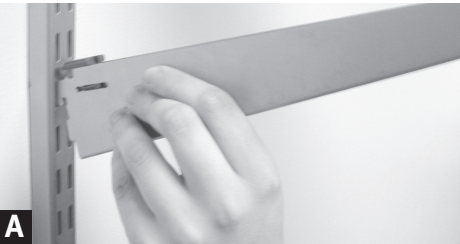
Insert brackets Insert brackets into uprights at desired locations. Note: Install brackets and shelving at the top first and work down. Brackets will not fit into upper two slots of each upright.
