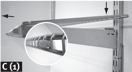
Install shelves into brackets Confirm that the bracket locks are unlocked and install shelving making sure that the "nose" of the bracket is projecting out through the front edge of the shelf. Note: For maximum weight capacity, do not insert brackets into bottom slots of upright.
