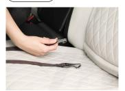
Attach lower LATCH fixings to the anchor points at the seat base. The fixing points may behind covers or where the seat back and base come together.
