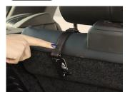
With both bottom straps attached, lift the top tether over the seat and attach to the rear seat LATCH point.
