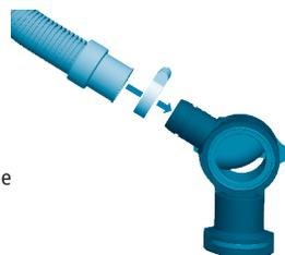
**IMPORTANT:** Hosing should follow a straight path from the filter to the aquarium rim, with no slack and no loops. If the hosing is too long, the filter will not work efficiently (the maximum length of the hosing is 6.5 ft / 2m).
