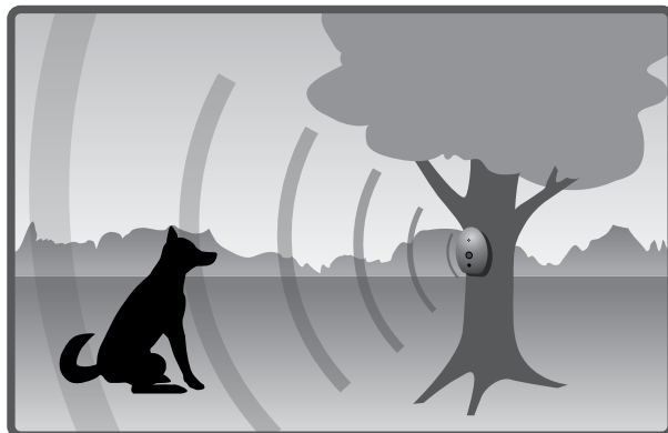
Mount to a tree using the mounting hole on the back of the unit
