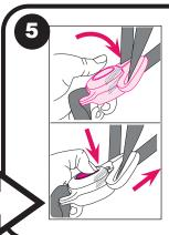
Unbuckle harness by tilting top of buckle down, press top of red button, and pull tongues out of buckle.
