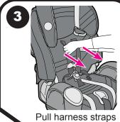
Pull harness straps hrough seat back and seat pad.
