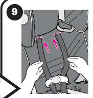
Re-insert straps through slots in seat pad and seat back.
