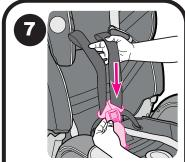
Slide NEW buckle onto harness straps. MAKE sure not to twist straps.
