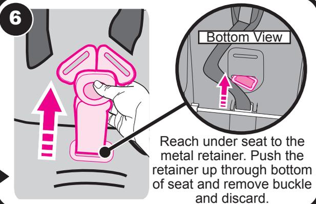
Reach under seat to the metal retainer. Push the retainer up through bottom of seat and remove buckle and discard.
