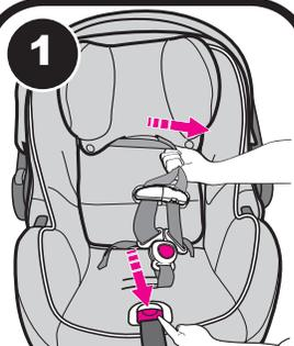
To loosen straps, lift lever and pull harness straps.
