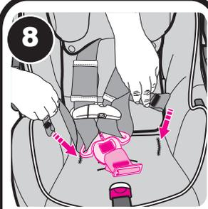
Insert waist straps back through seat pad and seat bottom slots.
