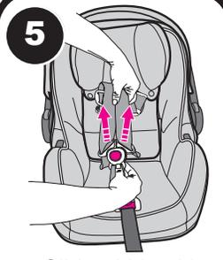
Slide old buckle assembly off of harness straps as shown.
