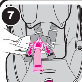
Slide NEW buckle onto harness straps from the front to the back. Depending on your buckle, the tongues may have "BACK" written on the back of tongue. MAKE sure not to twist harness straps.
