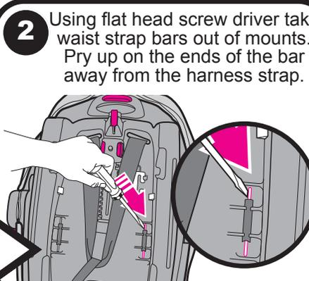
Using flat head screw driver take waist strap bars out of mounts. Pry up on the ends of the bar away from the harness strap.
