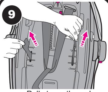
Pull straps through slots in seat pad and seat back.
