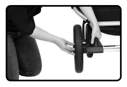
**1** To install, gently slide the rear wheel's axle into the hole in the frame until the wheel clicks into place.
