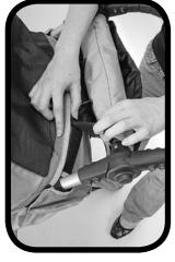
**4** Once canopy is in place, attach the console by aligning the velcro strips on the console and canopy.
