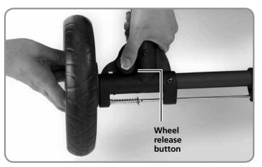
**1** Press the wheel release button while gently sliding the wheel away from the wheel mount.
