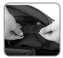
**3** Unfasten seat straps from around the bottom/back of the frame, located behind the front wheel.
