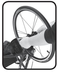
**3** Tighten by turning the wheel lever while holding the opposite side.
