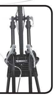
**2** Insert the front wheel into the forktips by aligning the axle flats with the forktip flats.
