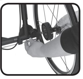
• *To install:* Gently slide the wheel's axle into the hole in the axle end until you hear it click into place.
