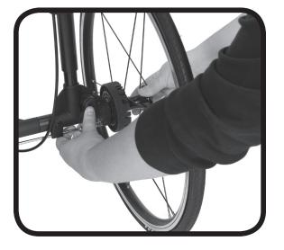
• To remove, simply press the wheel button while gently sliding the wheel away from the frame.
