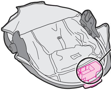
Remove bottom of seat pad and attach vibration unit onto center of curved seat tube with 2 screws. Replace seat pad.
