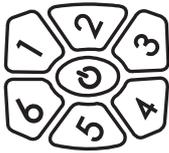
**SPEED** - Press On /Off button or press any speed from 1 to 6. When pressing On/Off button, it automatically starts with the last speed setting that was selected before the swing was turned off.
