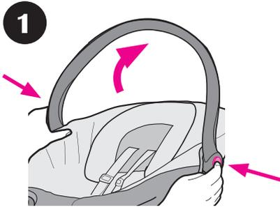
To lower, press handle adjustment buttons on both sides of handle and rotate back.
