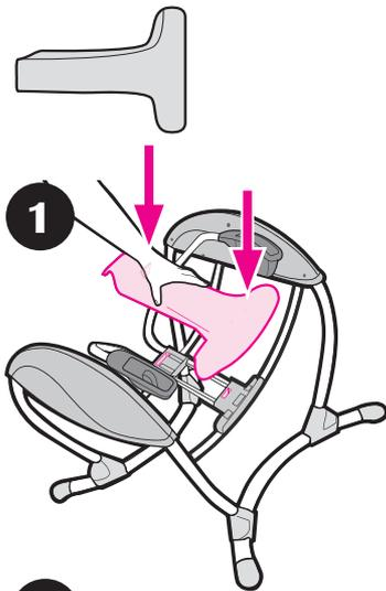
Attach plastic cover over tubes as shown until it snaps into place.
