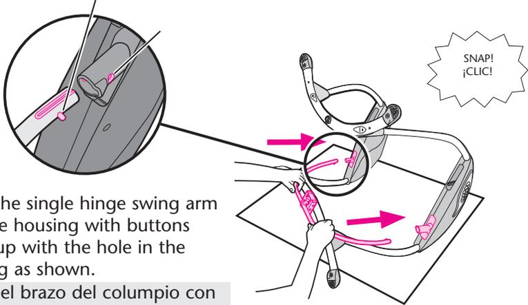
Insert the single hinge swing arm into the housing with buttons lining up with the hole in the housing as shown.
