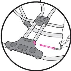
Insert a bolt through the holes in the swing arm bracket as shown. Tighten bolt with the wrench provided. Repeat with the other bolt on the other bracket.
