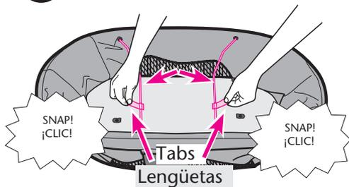
Rotate wires on both sides of bassinet down until they snap under plastic tabs. Repeat on other side as shown.
