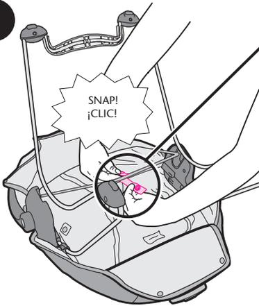
Pull snaps over the wire and fasten together.
