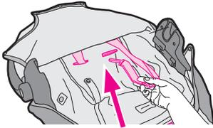
To change harness strap position, unfasten snaps on bottom of seat to reach the harness straps. Pull harness straps out of slots in seat pad.
