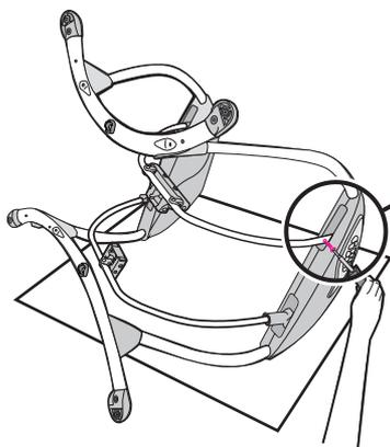
Fasten the screw as shown into hanger mount.
