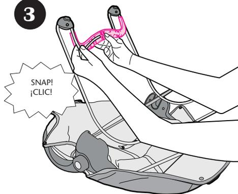
Insert leg wire into leg brace as shown until it snaps into place.
