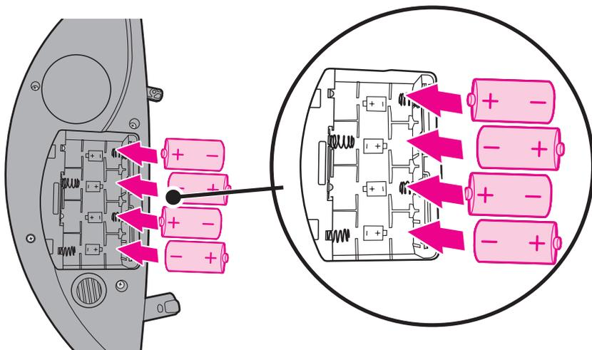
**With baby out of swing,** open the battery compartment lid by inserting a key into the slot. Insert four D (LR20 -1.5V) batteries. Replace battery lid.
