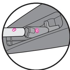
Attach hanger tube with double hinge until the buttons snap into place as shown.
