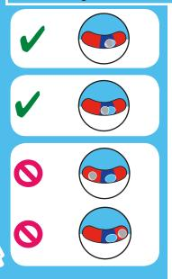
Vehicle **MUST** be on level ground.
