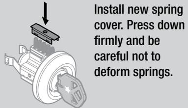
Install new spring cover. Press down firmly and be careful not to deform springs.
