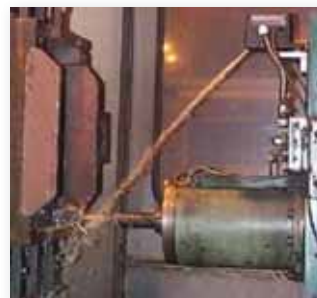
Inadequate coolant delivery
