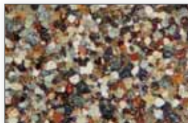
Microstructure of \alpha -alloy Ti5Al2.5Sn.
