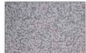
Alpha-beta alloy Ti6Al4V showing primary alpha grains and a fine alpha-beta matrix structure.
