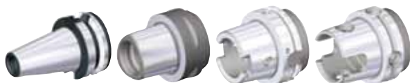
Fig. 1 The various spindle connections commercially available today: 7/24 ISO taper, KM (ISO TS), HSK, and PSC.
