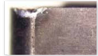
Kennametal's CNGG-432FS KC5510 Tool life: 26.5 minutes
