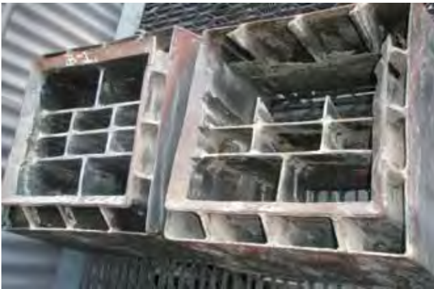
Side by side comparison (boiler side view) of the weld overlay protected coal nozzle tip (right) and the Kennametal Conforma Clad tip (left).
