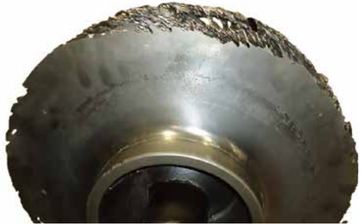
Pump impeller after 13 months without Conforma Clad protection
