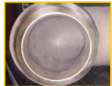
Return Bend Ready for Installation
