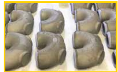
Clad Return Bends Ready for Sintering
