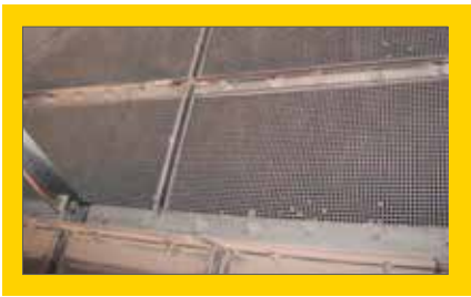
Conforma Clad screens after nine months.
