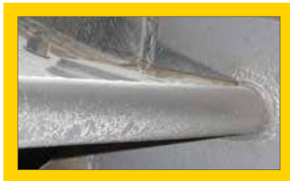
Fan blade protected with Conforma Clad liner.
