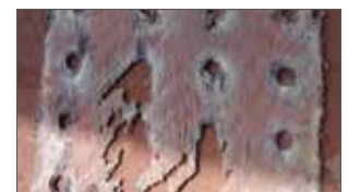
Chrome carbide fan blade after three months.
