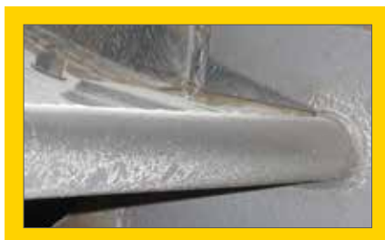
Fan blade protected with Conforma Clad liner.
