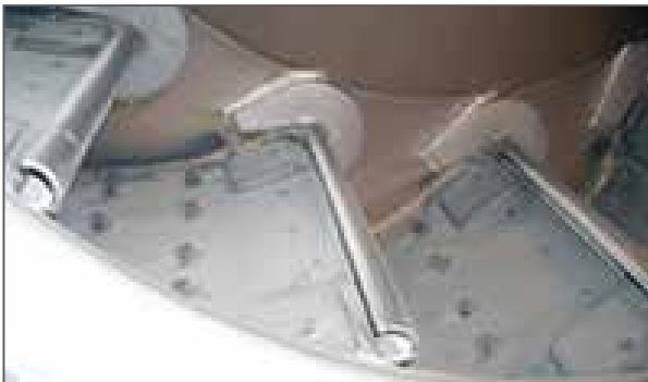
Leading edge and center plate protection.
