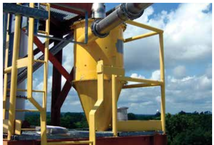
Cyclone clad with Kennametal infiltration brazen tungsten carbide wear protection.
