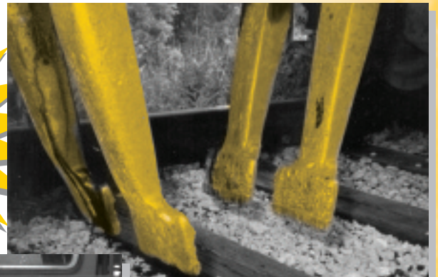
Railroad tamping tool with KenCast protection.
