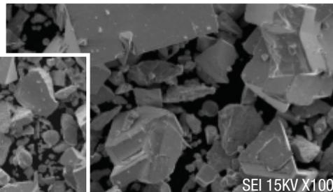
The Kennametal macrocrystalline thermit process provides a highly effective method for the production of tungsten carbide crystals directly from ore concentrates. Unique properties of macrocrystalline WC are being exploited in many special applications, including diamond tool matrix powders. WC crystals grown to 500 microns in an iron menstruum, with a stoichiometric 6.13% carbon, yield a stable carbide ideal for infiltration and wear applications.
