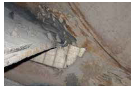
Fan blade protected with chrome carbide weld overlay liner.
