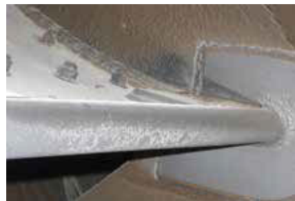
Fan blade protected with Conforma Clad liner.
