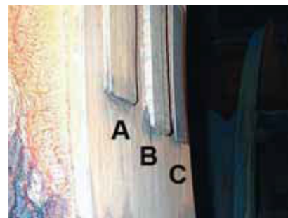
Port Alberni Wear Protection Test Results — A. Alloy Steel; B. Chrome Carbide Weld Overlay; C. Conforma Clad Brazed Tungsten Carbide Cladding
