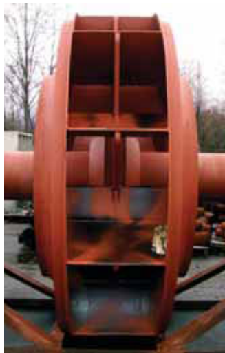
Port Alberni's ID fan protected with Kennametal Conforma Clad infiltration brazed tungsten carbide cladding.
