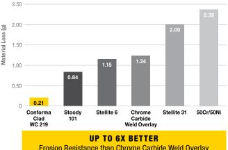
**Erosion Resistance than Chrome Carbide Weld Overlay**
