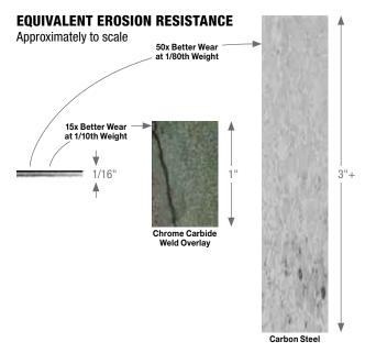
One sixteenth inch (1/16") of Kennametal's Conforma Clad tungsten carbide wear protection performs 15x better against erosive wear than an equivalent layer of chrome carbide weld overlay and 50x better than carbon steel. Because of its extremely high metallurgical bond strength, the cladding is up to 5x more erosion resistant than typical nickel chromium alloy castings alone.
