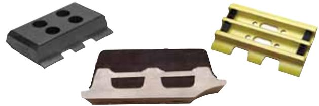
CUSHOTRAC™ Mold-On Bodenplatten
