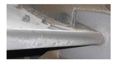
Kennametal's Conforma Clad™ tungsten carbide claddings have been cited by the Electric Power Research Institute as the most resistant of approximately 30 materials evaluated in fly ash erosion tests.
