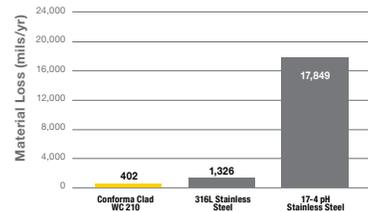
ASTM G31 testing shows Kennametal's WC 210 provides superior corrosion resistance.
