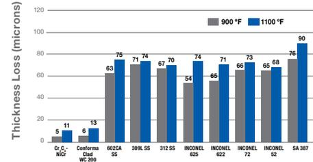
EPRI testing at elevated temperatures confirms that Kennametal's WC 200 protects boiler tube applications from erosive wear better than other accepted alternatives.
