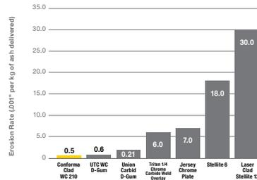
EPRI testing found that Kennametal's WC 210 provides superior erosion protection for power boiler fan blades exposed to high-velocity bituminous coal fly ash.
