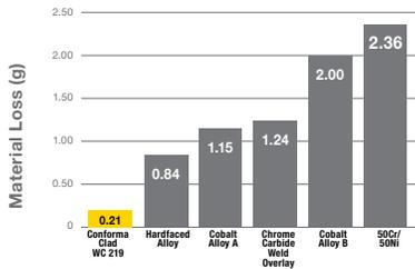
Laboratory testing, following ASTM G73 standards, on low swirl coal spreaders determined Kennametal's WC 219 provides the best erosion protection from fine grit black beauty coal slag.
