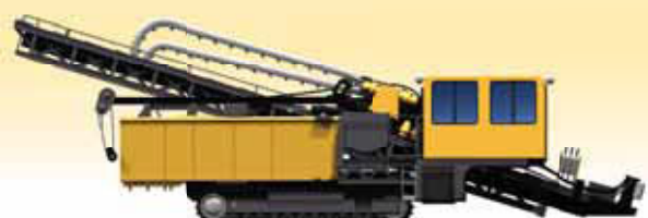
Horizontal Directional Drilling
