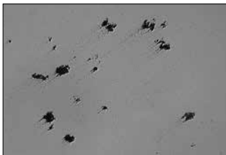
Pitting corrosion on all faces.
