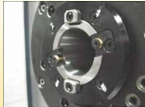
Taper face tool's axial position is maintained even at high rotational speed.
