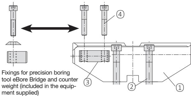
Fixings for precision boring tool eBore Bridge and counter weight (included in the equipment supplied)
