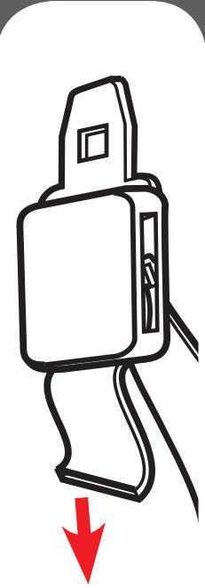
Grab the sides of the seat at the belt path and slide the seat side-to-side and front-to-back. The seat should not move more than 1 inch (2.5 cm).
