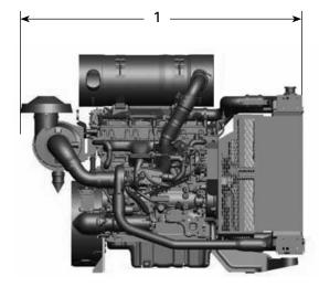
(1) Length — TA: 1433 mm (56.4 in) TTA: 1433 mm (56.4 in) (2) Width — TA: 820 mm (32.3 in) TTA: 795 mm (31.3 in)
