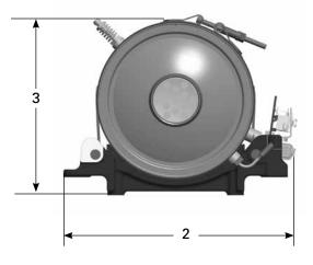
Less than or equal to 82 bkW (110 bhp) 244.9 mm (9.6 in) DIAMETER BASE CONFIGURATION Approximate Size and Weight (1) Length — 802.5 mm (31.6 in) (2) Width — 365 mm (14.3 in) (3) Height — 279 mm (11 in) Weight — 34 kg (75 lbs) *Greater than 82 bkW (110 bhp)*  **270.3 mm (10.6 in) DIAMETER BASE CONFIGURATION Approximate Size and Weight** (1) Length — 828 mm (32.6 in) (2) Width — 365 mm (14.3 in) (3) Height — 300.5 mm (11.8 in) Weight — 37 kg (81.6 lbs)
